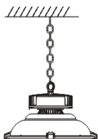
Hanging chain installation
